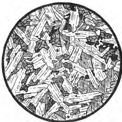
FIG. 32. Diabasic texture, drawn from a microscopic slide of a diabase from Figeon Pt., Minn. The actual field was three eighths inch (1 cm.). The rods of plagioclase are shown enclosing the augite olivine and magnetite. The shaded mineral with light borders is augite; the shaded mineral with heavy borders is olivine. The black mineral is magnetite.
